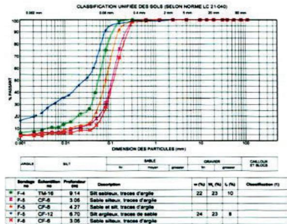
Figure 6 - LOGES 3 - Compacsol performance boreholes samples from conditioned soil
